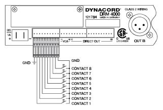
As shipped, the configurations of the eight control inputs have been factory-pre-programmed for using the DRM 4000 in a multitude of applications. For further detail, please refer to chapter 8 and to the additional information sheet "DRM 4000 FACTORY CONFIGURATION".
